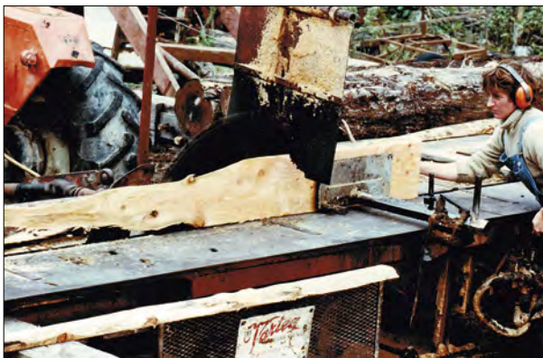
Below: Sarah milling the timber for the house. Unlike today's portable mills this one was physically demanding, but way superior to the first one we had in 1972
